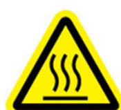
Burn Hazard / Hot Surface
