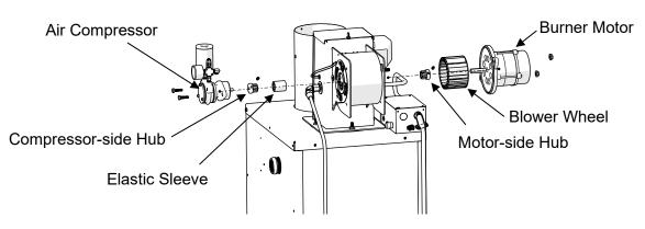
13. Run the burner and confirm/adjust the air pressure to 3 - 4 psi.
