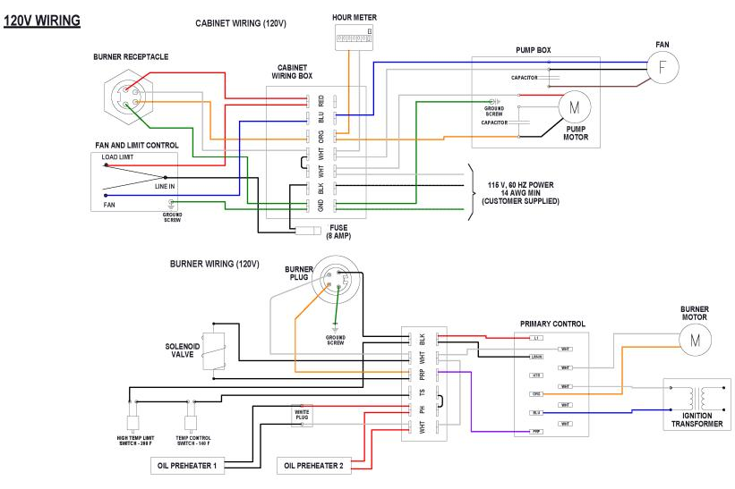
ITEM: 98120083 - WIRING DIAGRAM, 75H (REV B - CARLIN PRIMARY CONTROL) RELEASED: 03/11/2021
