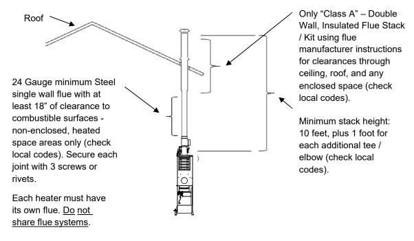
Installation of Vertical Flue
