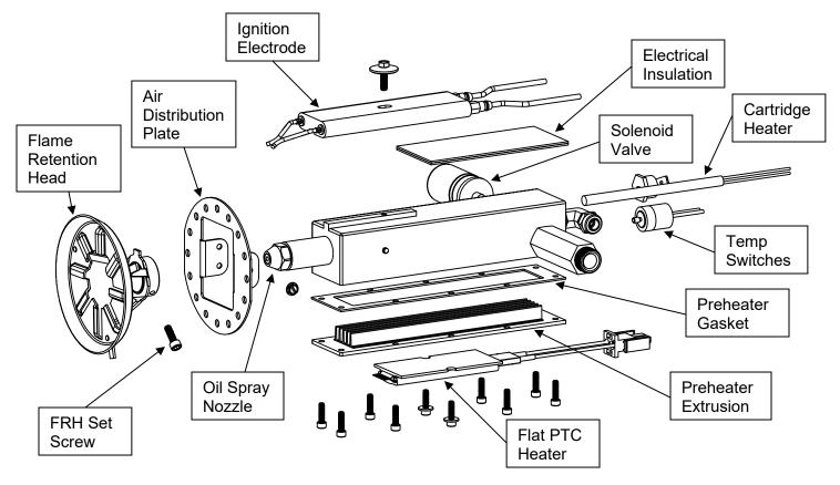
Nozzle Line Assembly – Exploded View
