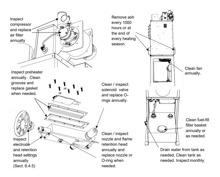
**ACAUTION** Always wear personal protective equipment when performing inspection and service. The maintenance schedule is the minimum recommended, but if you see smoke or have trip outs then the unit must be shut down and serviced immediately before running it again. Increase the maintenance as your situation requires.
