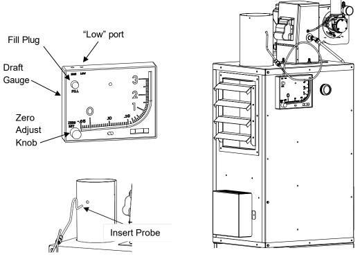
**Draft Gauge and Probe Installation**
