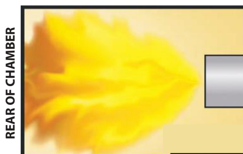
Flame is over-fired
