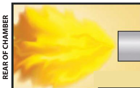
Flame is over-fired
