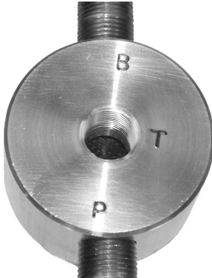
Bottom View of the Aluminum Oil By-Pass Regulator
